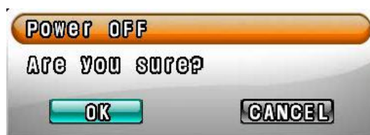
[Fig.6-2 Message of POWER off]
